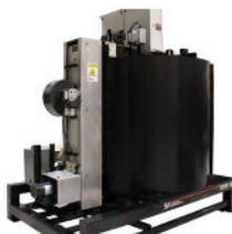
Rear view — blower exhausts hot air and ozone from the curing chamber.
