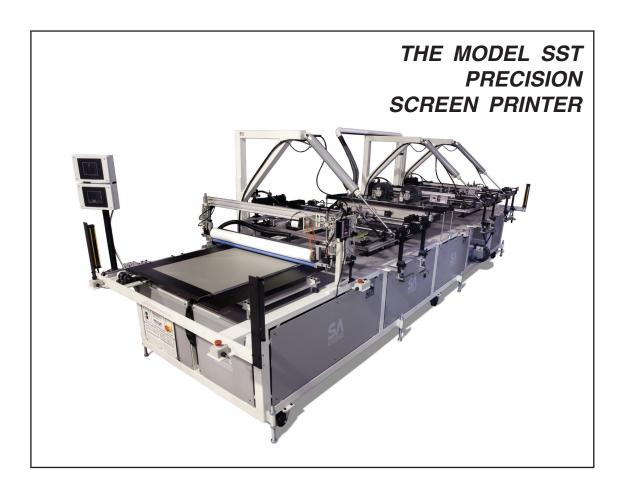
The Model SST can screen print up to six colors in one machine cycle with super precision accuracy, at an affordable price. The SST is the only screen printing machine in the world that allows you to change the sequence of color laydown without moving screens, squeegees, or flood bars. Automatically double or triple print color with the user friendly touch screen interface. You can also precisely set individual curing exposures and do it all with one UV light source.
