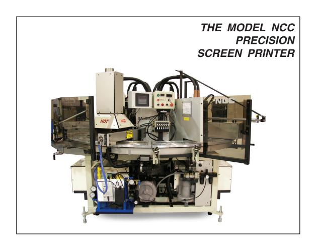
The model NCC Screen Printer (U.S. Patent # 5,784,932), a great innovation which delivers superior performance. The NCC is designed for unrivaled speed and exceptional productivity. Speeds variable to 3600 cycles per hour (depending on article) are easily achieved.
